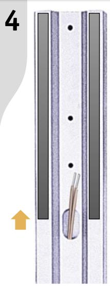
Thread Speaker Wires Cut speaker wire 4 to appropriate lengths for all speaker connections and set aside. Place each long stand upright on its base. Thread main speaker wire through oval opening on stand and pull through opening on underside of base. Pull wire all the way through leaving extra length near oval opening as shown. Attach color cable tags to all speaker wires as shown in Step 10. Apply non-skid pads on stands.
