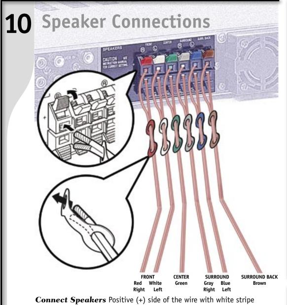
attaches to (+) terminal. Negative (-) side attaches to (-) terminal. Attach appropriate colored cable tags as shown.
